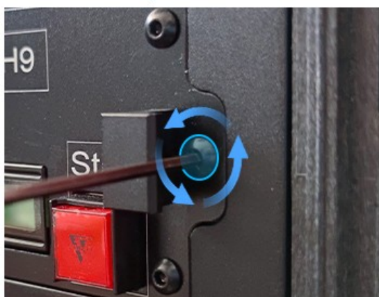
The jammer module can be quickly replaced by removing the hexagonal screws on both sides
