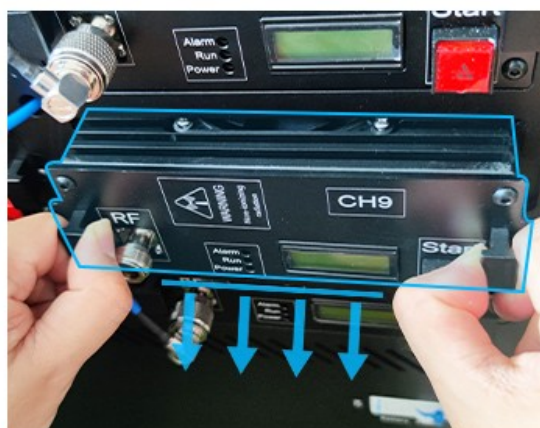
The jammer module can be quickly replaced by removing the hexagonal screws on both sides
